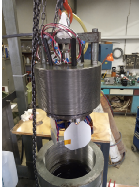
Figure 37: Pressure testing of the penetrators.
